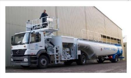
A semi-articulated refueller incorporating a 4x2 chassis and single trailer axle configuration for optimal manoeuvres on the airport ramp. The elevating platform and refuelling unit are mounted on the chassis unit immediately behind the cab, with the semi-trailer tank attached by means of a liquid 5<sup>th</sup> wheel. The refueller is designed and constructed in accordance with the latest European Standards BS EN 12312-5 and JIG 1 Issue 11 requirements where applicable.
